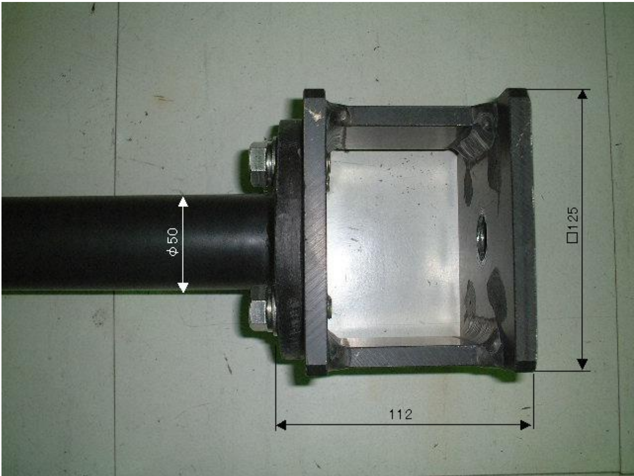
Figure 2-7 I/F on Illuminometer Supporting Pole
